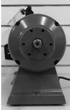
Remove the grinding wheel and guard off the side of the bench grinder that you would like to install the linishing attachment to. Keep the original nut and washer holding the grinding wheel in place
