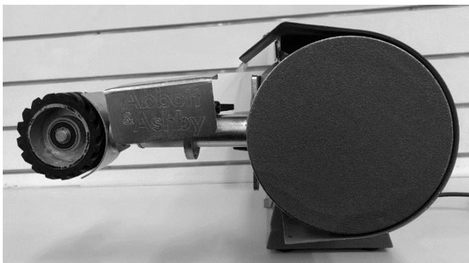
Attach the abrasive disc (C) to the backing plate. Hold firmly for a few seconds to ensure the adhesive activates.
